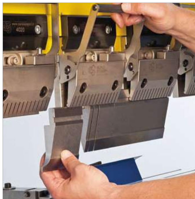
Quick-release mechanism for stamp
