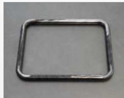
3/4" steel pipe as framework
