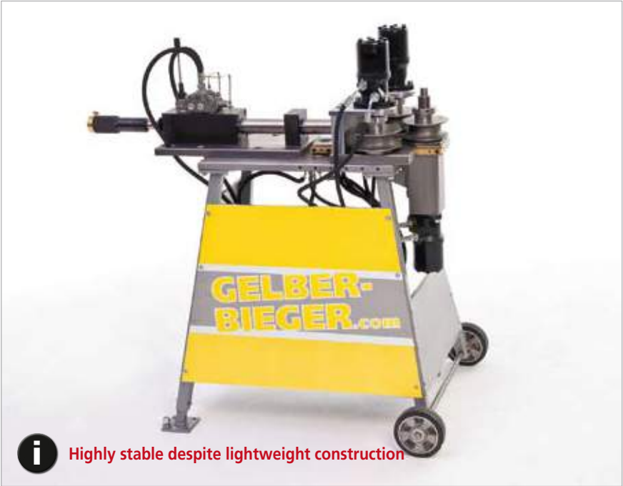
Vario 2 3 hydraulic feed and 3 motorised rollers
