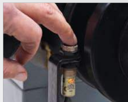
Proximity switch determines the start of the programme
