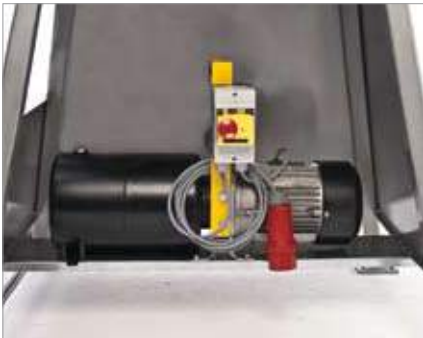
Integrated hydraulic unit
