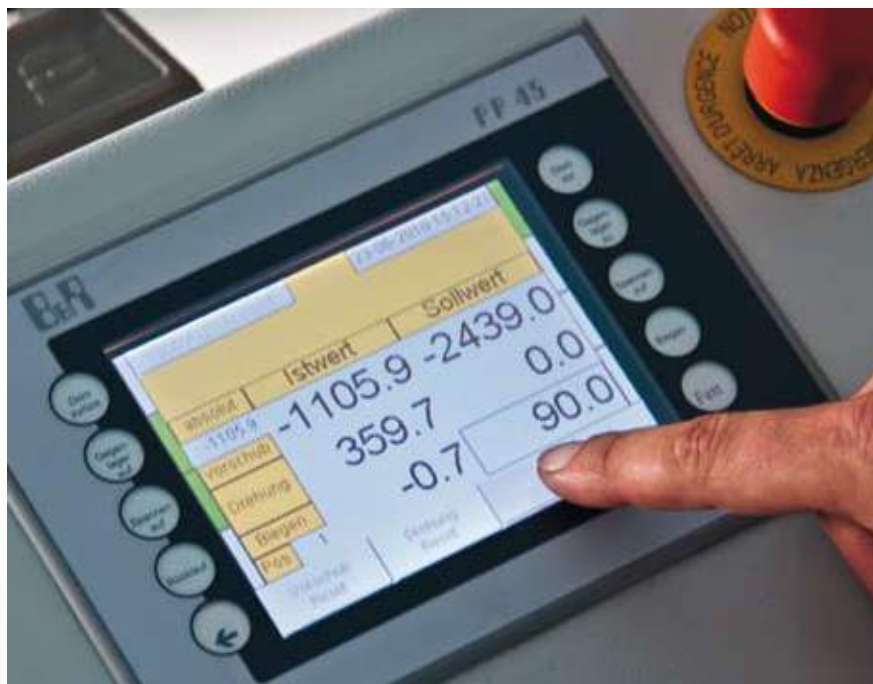
Touchscreen onboard control panel
