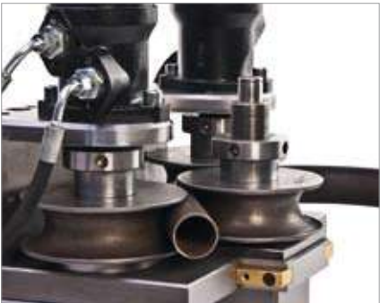
Bending capacity for tube diameters of up to 48 mm
