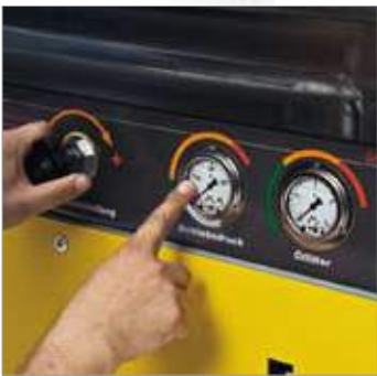
Pressure adjustment up to 300 Bar
